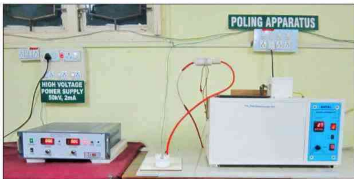
Poling Apparatus with High Voltage Power Supply
